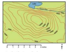
The closer the lines are together, the steeper the slope.
